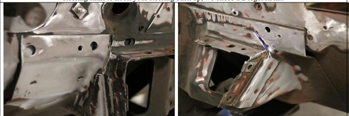
Prep the firewall mounting surface by removing the small flaps on both the driver & passenger side. Pictured above is what it should look like after the top layer (flap) has been removed.
