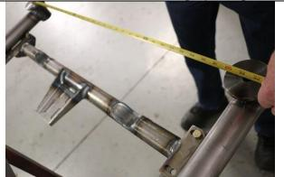
The rear frame rails pull together after the clip is removed from the weld fixture. To facilitate installation and proper alignment, spread the rails and temporarily install the transmission crossmember with the bolt hole centers at 33.5 inch. Once the suspension clip is installed and all bolts tightened, you can remove the crossmember.
